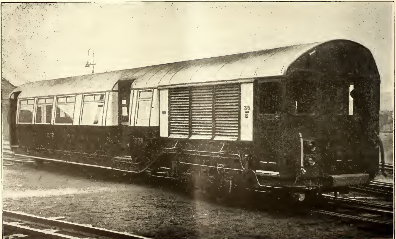
LONDON UNDERGROUND EXTENSION—MOTOR CAR WITH CONTROL EQUIPMENT COMPARTMENT ELEVATED TO CLEAR MOTOR TRUCK
